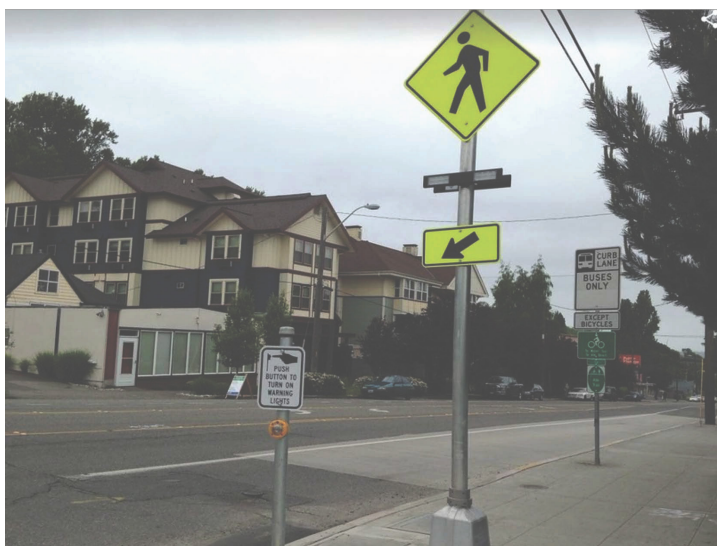
An example of a rectangular rapid flashing beacon, along with a button on a post
