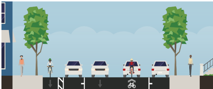
Uphill PBL/downhill sharrow concept (26th Ave to Martin Luther King Jr Way, facing east)
