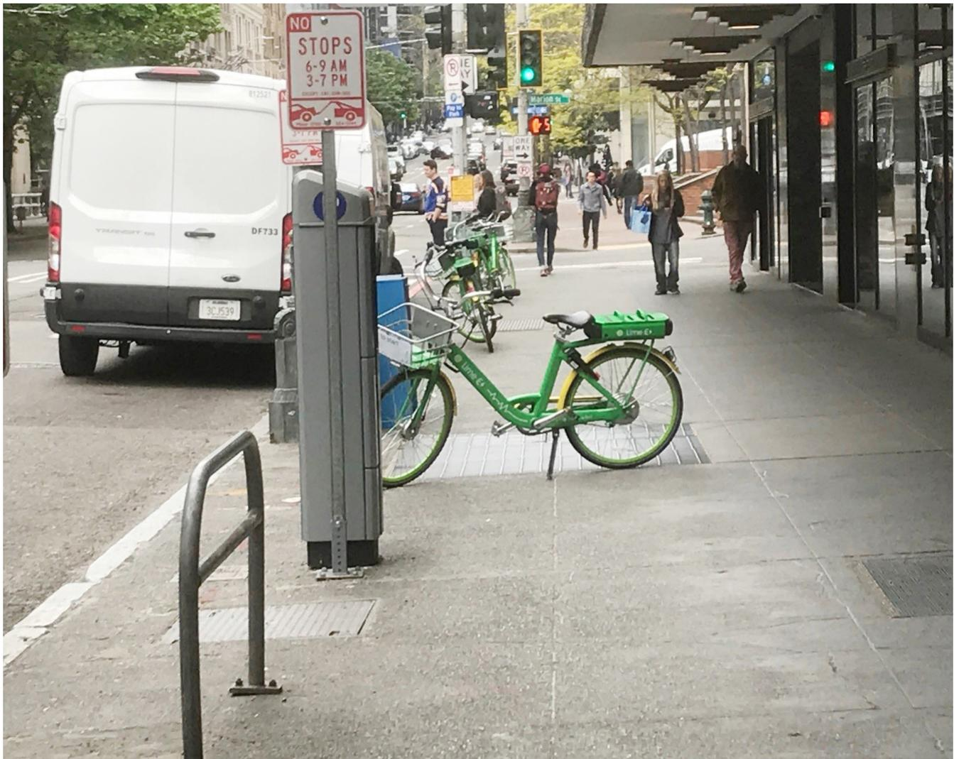
Figure 2: This bicycle blocks the sidewalk and is categorized as an obstruction hazard. It does leave over 4' of passage so is not an ADA-prohibited obstruction hazard.
